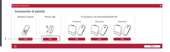
2. Once the searching pop-up appears, press the pairing button on the accessory with a small pointed object such as a pen tip or paper clip. Follow the pairing instructions displayed.
