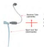
The sport lock tail and the receiver tube should be going in opposite directions.
